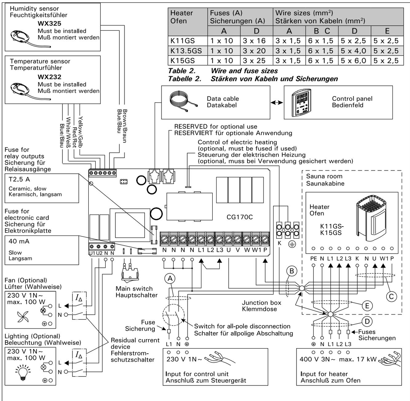
**Figure 6. Electrical connections (K11GS-K15GS)**
