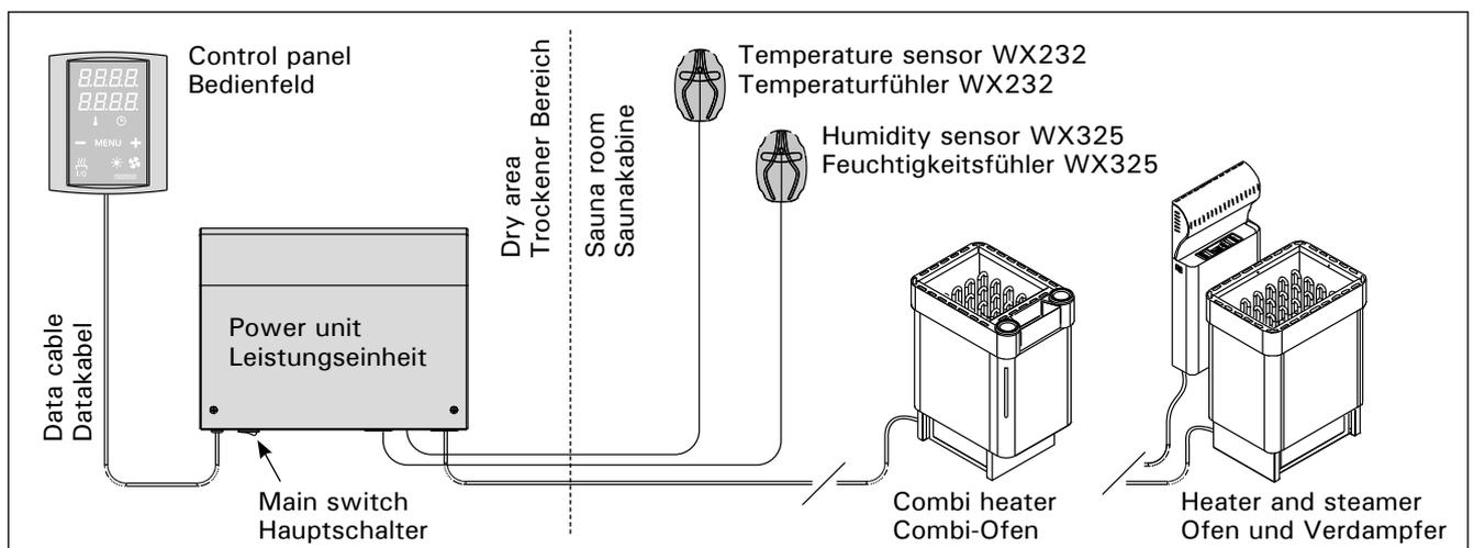
Figure 1. System components
