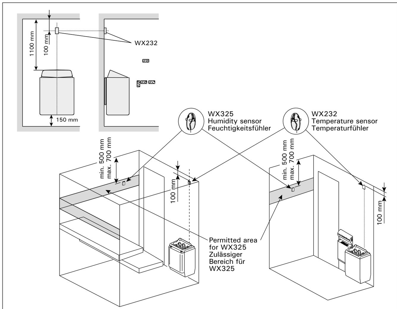
Figure 8. The place of the temperature and humidity sensors in connection with wall-mounted heaters
