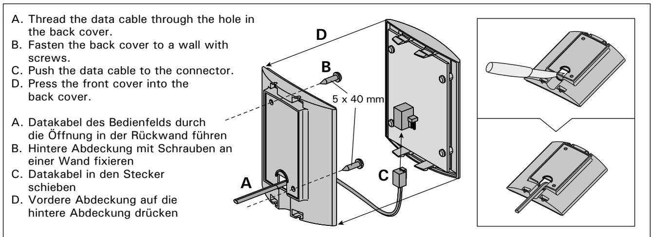
Figure 4. Fastening the control panel
