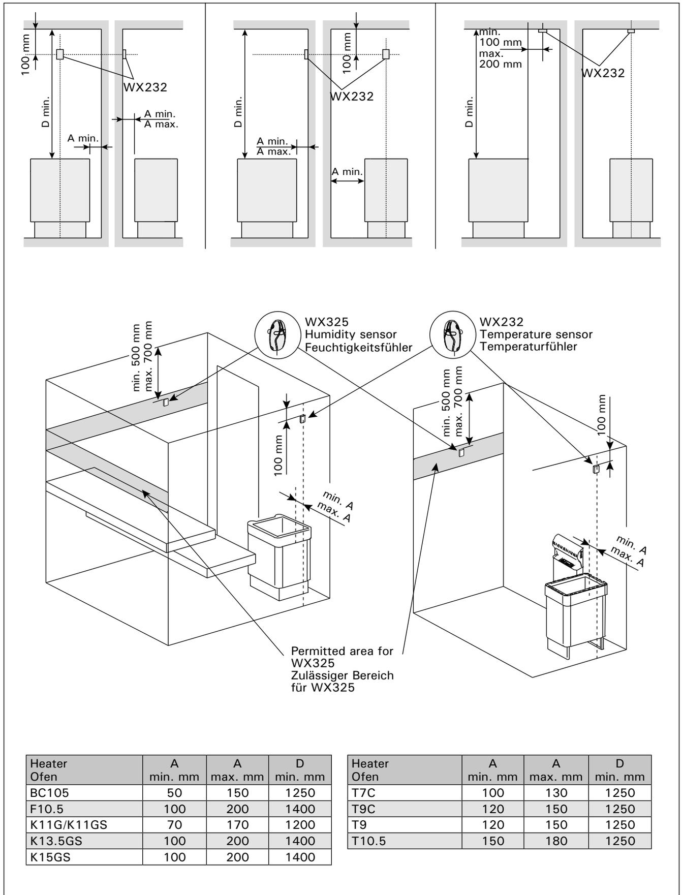
Figure 9. The place of the temperature and humidity sensors in connection with floor-mounted heaters
